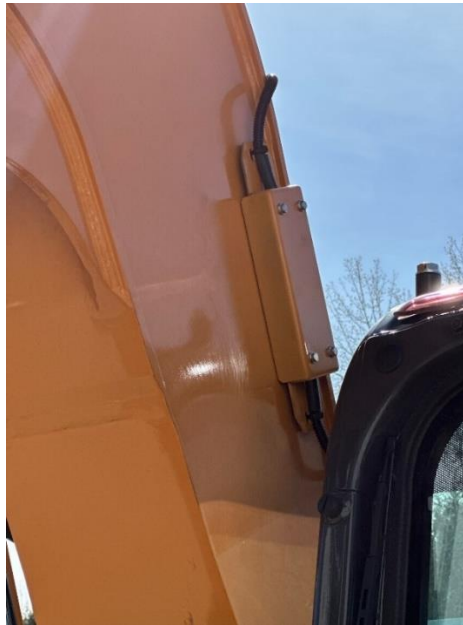
Figure 2-12: Boom sensor mounted to boom top showing plate welds
