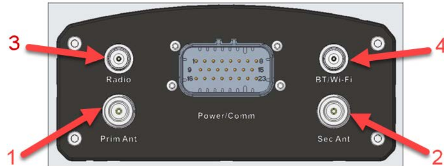
Figure B-2: VR1000 pin-out assignments
