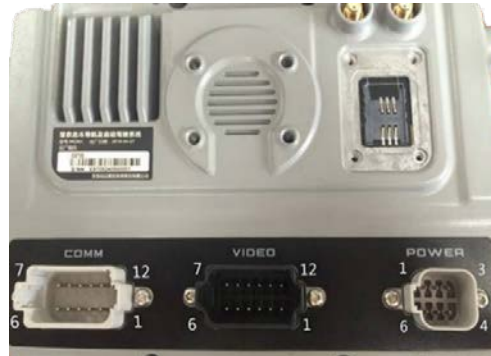
Figure B-3: IronOne pin-out assignments
