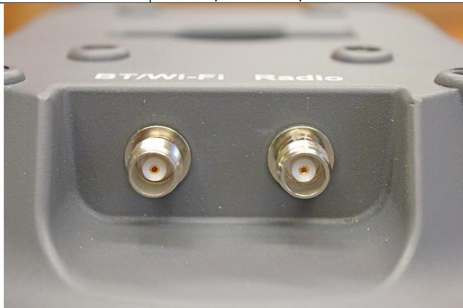
**Figure 3-14: UHF antenna connections**
