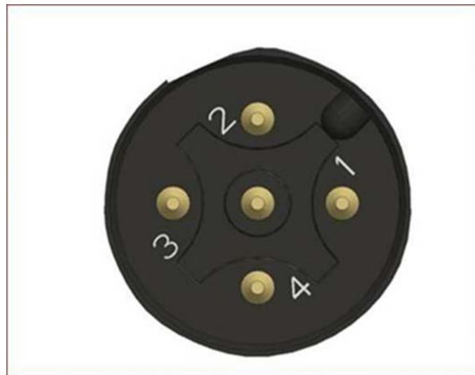
Figure 2-11: 5-pin (male) CAN port pin-out
