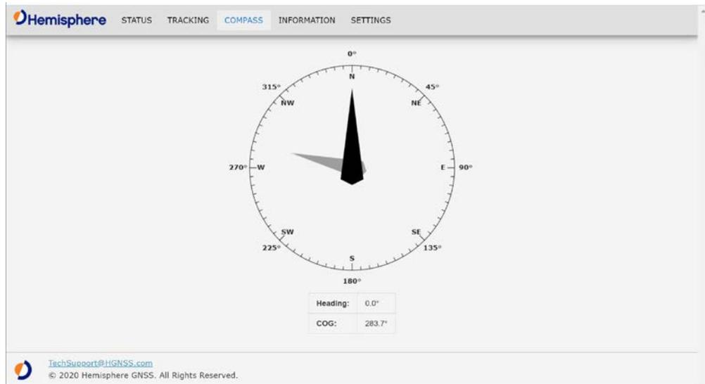
**Note:** The provided V200s Smart Antenna heading will only provide a stable indication if the receiver is moving.
